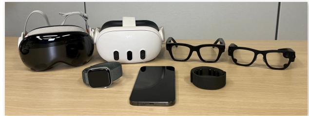
Figure 5: Different AR display and input devices used in our prototypes. From left to right, the first row shows Apple Vision Pro, Meta Quest 3, Meta Ray-Ban Display, and Meta Project Aria glasses; the second row shows Apple Watch, iPhone, and Meta Neural Band.
